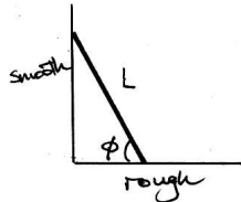
Figure 2.5: Ladder leaning against the wall. The surface between the ground and the ladder is rough while that between the ladder and the wall is smooth.
