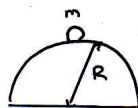
Figure 6.1: A ball resting on top of a hemisphere of radius R . The ball is given a small horizontal perturbation.
