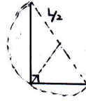
Figure 2.17: By considering the ladder as the diameter of the circle, circle geometry gives that the string has a length equal to the radius of this circle (the reference is converse of \angle in semicircle).
